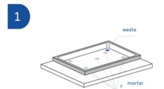
Position the waste according to the existing drain hole and according to the position in the bathroom. Supporting points should be made using low water mortar alongside the corners as well as the centre.
