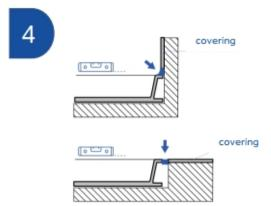
Verify the right horizontal positioning by means of a spirit level.
