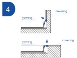
Verify the right horizontal positioning by means of a spirit level.
