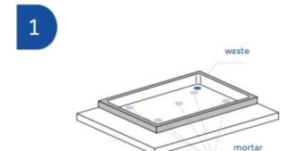
Position the waste according to the existing drain hole and according to the position in the bathroom. Supporting points should be made using low water mortar alongside the corners as well as the centre.
