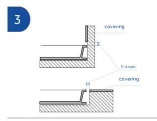
Position the shower tray paying attention to the thickness of the covering (or to the floor thickness in case of recessed installation) and leaving a gap of 3-4 mm.
