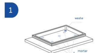
Position the waste according to the existing drain hole and according to the position in the bathroom. Supporting points should be made using low water mortar alongside the corners as well as the centre.
